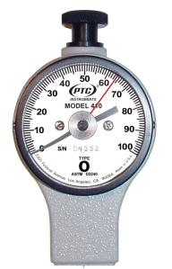
ASTM Type O Durometers measure the hardness of soft printing rollers, nylon, rayon, orlon, artgume, and textile windings.
