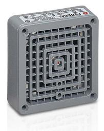
Model 350 Vibratone® Horn produces a loud tone by the electro-mechanical vibration of a diaphragm. Its compact size, loud output and heavy-duty construction makes the 350 ideal for industrial and institutional signaling applications. It's popularly used for general alarming, start and dismissal noticing, coded paging and process control in noisy areas.
