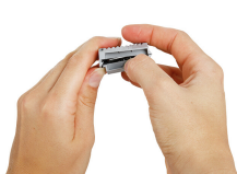
Open the Gelbox at the side latches.
